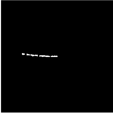
Fig. 14 Image from Fig. 13 has been binarized at multiple levels, and large areas have been identified. The image has been dilated one iteration.
