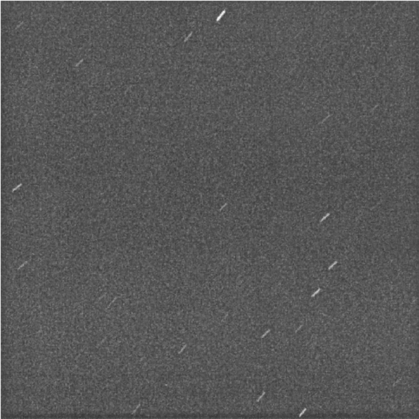
Fig. 2 Simulated star image ( \delta = 37 deg, \alpha = 191 deg) contrast enhanced. The camera was slewing 28 deg/s cross boresight. The camera configuration is similar to the configuration in Fig. 1.
